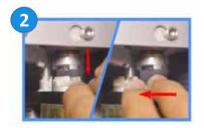
Separate the motor assembly from the coupling sliding the assembly down. Then pivot it towards the hand wheel.
