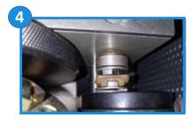
If the plastic motor coupler does not line up with the upper hub, use the hand wheel to put it into place
