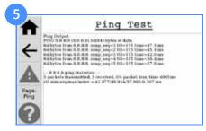
Read the output of the test. If the 2nd to last line reads '5 packets transmitted, 5 received, 0% packet loss' then the controller is successfully connected to the internet
