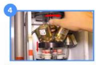
Spin the hand wheel to the right to lower the manifold.
