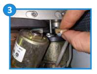
Remove the old plastic coupler and place the new one in. Make sure to center it on the metal hub.
