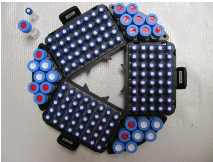
Figure 4-6. Photograph of sample vial configuration in the autosampler of Thermo Scientific/Dionex ICS-5000 + system with three 40-vial sample trays and three eight-vial calibration/QC standard trays.
