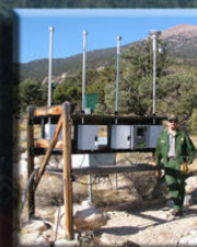
outside mounting on a rack built expressly for the IMPROVE samplers
