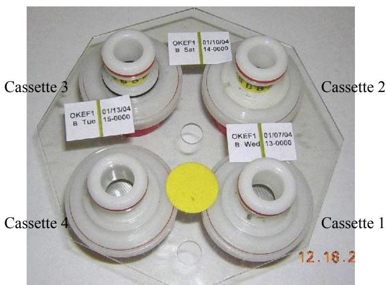
Figure 2-3. Sample cartridge for the 2B module (yellow sticker) with four cassettes. Only three of the cassettes contain sample filters (indicated by the three labels).
