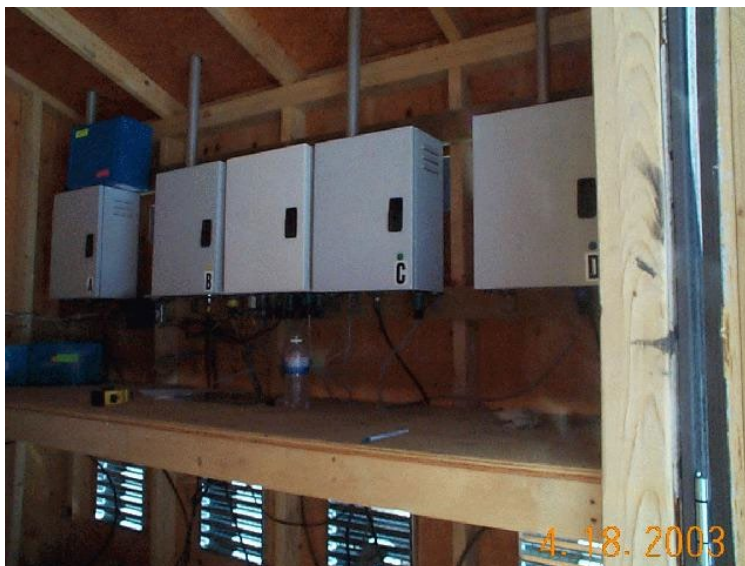
Figure 1-1. Photo of the IMPROVE aerosol sampling modules inside a shelter.
