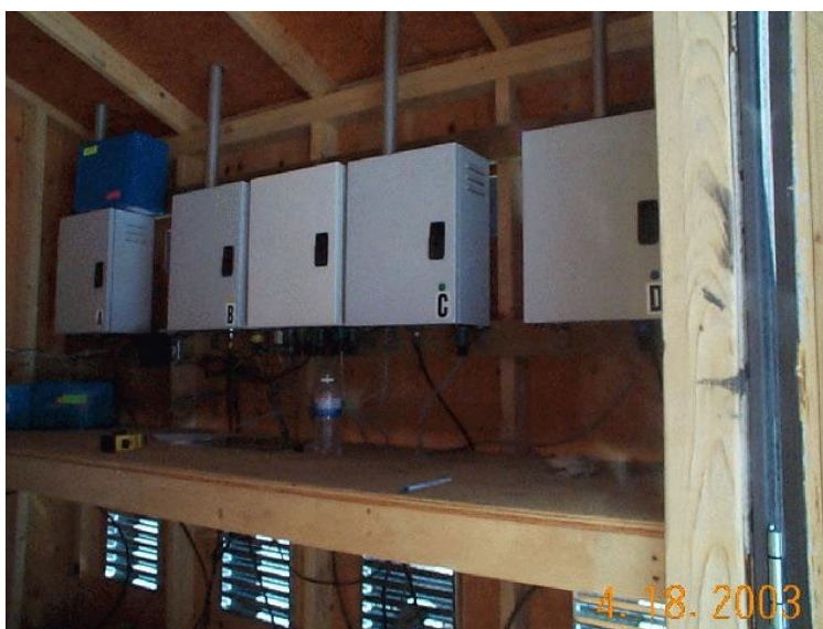
Figure 1. Photo of the IMPROVE aerosol sampling modules inside a shelter.
