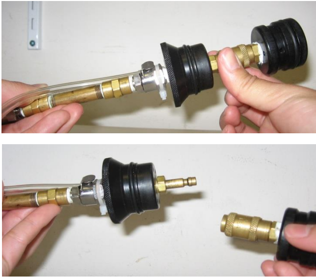
Figure 4. Releasing the probe plug.
