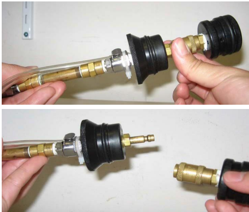
Figure 4. Releasing the probe plug.
