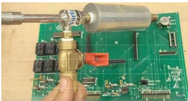
Figure 11. Thermostat Being Cooled with a Vortex Tube
