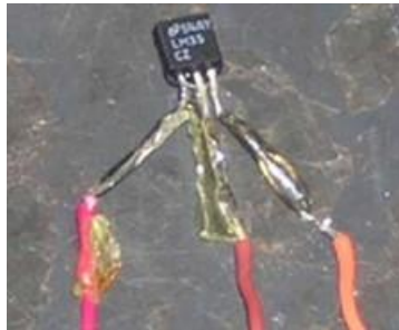
Figure 24. Wires in Order from Left to Right: Red, Brown, Orange.
