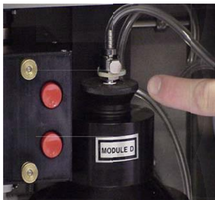
Figure 6. Placing the Probe in Module “4D” (con.)
