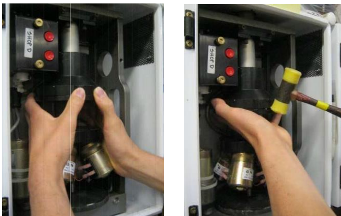
Figure 7. Removing the Bottom Lid of Module “4D”
