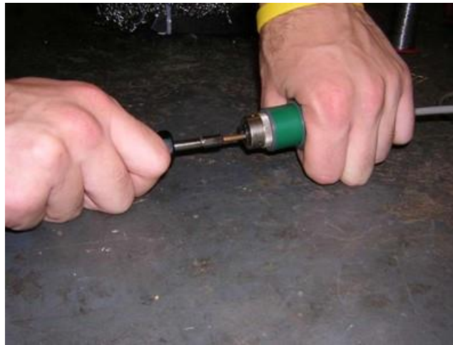
Figure 28. Removing the Connector Pins.
