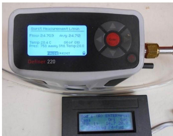
Figure 4. Operating the Definer 220
