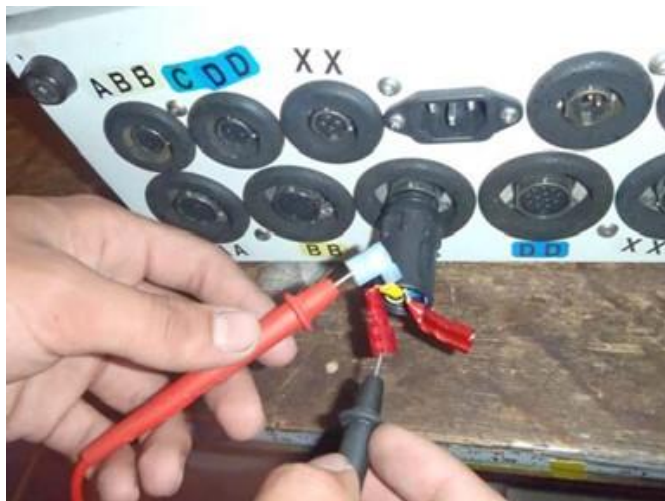
Figure 2. Checking 12V and 24V Sources.
