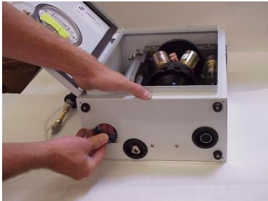
Figure 1. Removing the Plastic Cap and Stack Plug
