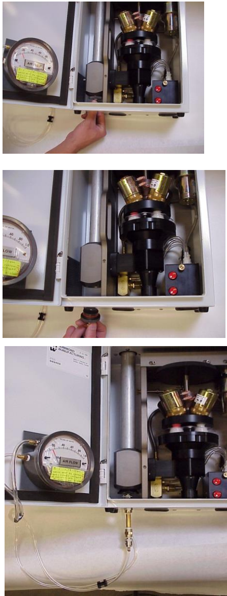
Figure 2. Inserting the Probe into the Tee
