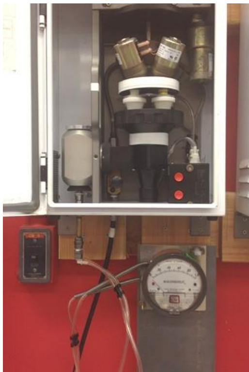
Figure 6. Calibration System with Magnehelic Flow Meter.
