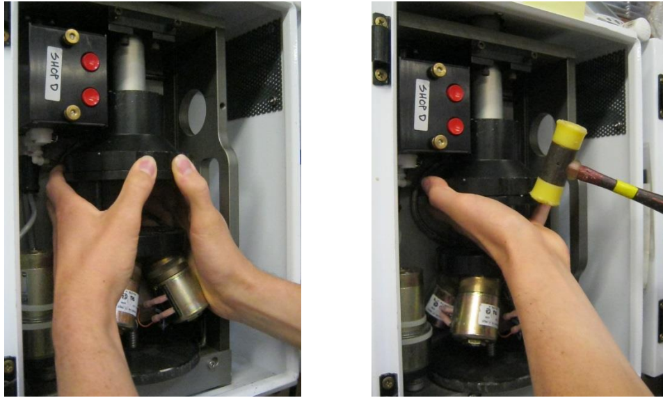
Figure 7. Removing the Bottom Lid of Module “4D”
