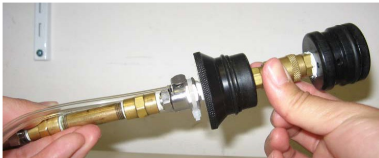
Figure 4. Releasing the probe plug.
