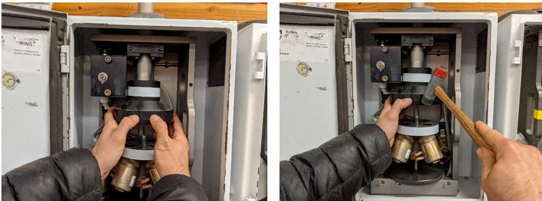
Figure 8. 4D O-Ring between stack and funnel.
