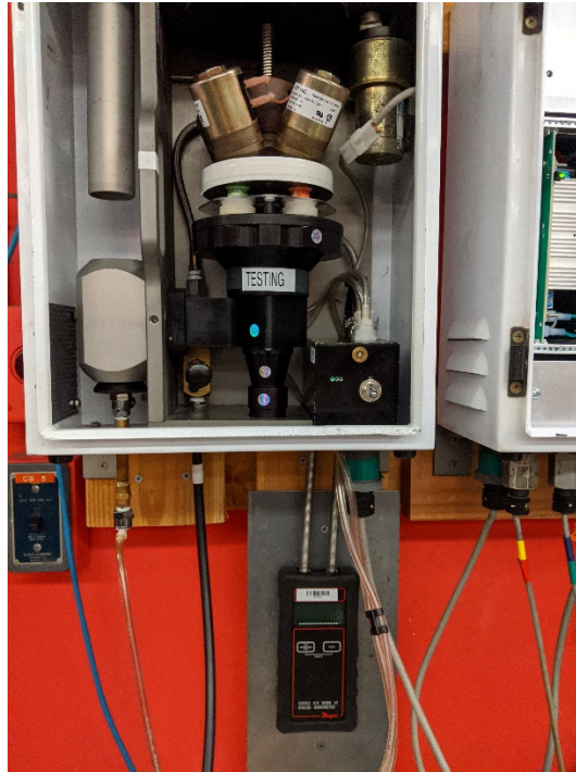
Figure 6. Calibration system with magnehelic flow meter.
