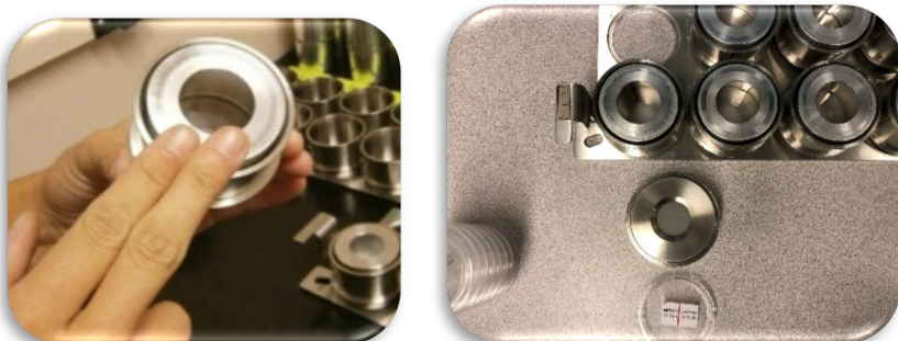
Figure 8. Sample holder cup handling and positioning.
