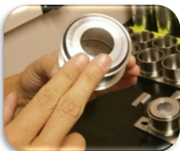
Figure 8. Sample holder cup handling and positioning.
