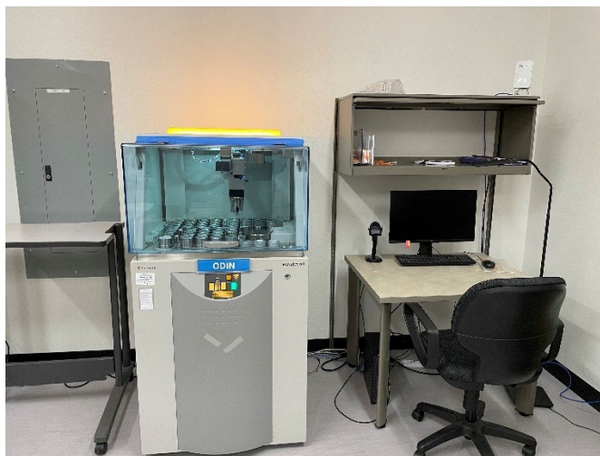
Figure 1. PANalytical Epsilon 5 analyzer and computer station in the XRF Laboratory at AQRC.
