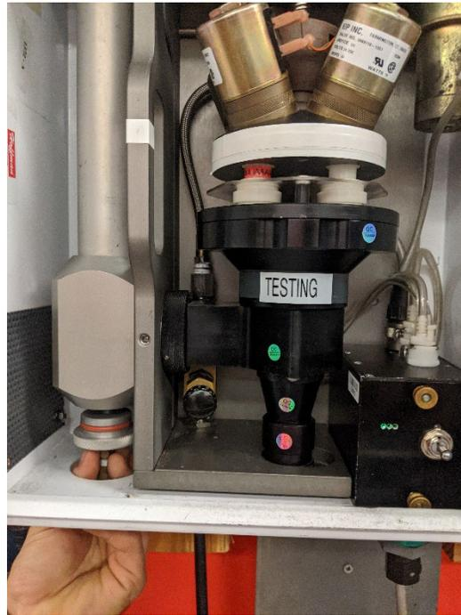
Figure 2. Inserting the probe into the tee.
