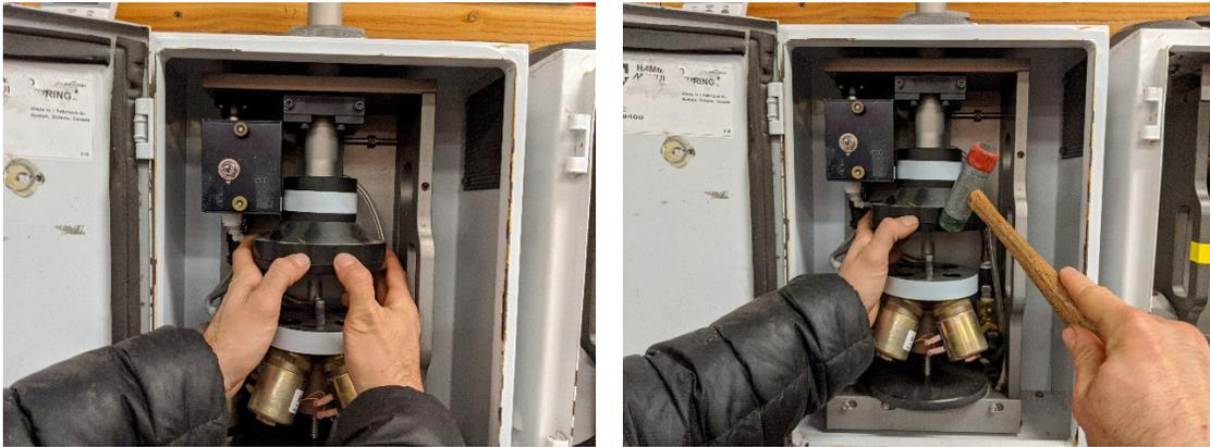
Figure 8. 4D O-Ring between stack and funnel.
