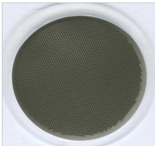
**Figure 1.** Photograph of an ambient fine particulate matter sample collected on a 25-mm polytetrafluoroethylene membrane filter (stretched across a polyolefin ring) in the IMPROVE network. This sample has the typical sample geometry (area, edges, and pixilated pattern) found in deposited particulate matter on filters used for X-ray fluorescence analysis. A support screen located downstream of the filter in the sample holder produces the pixilated pattern on the filter.
