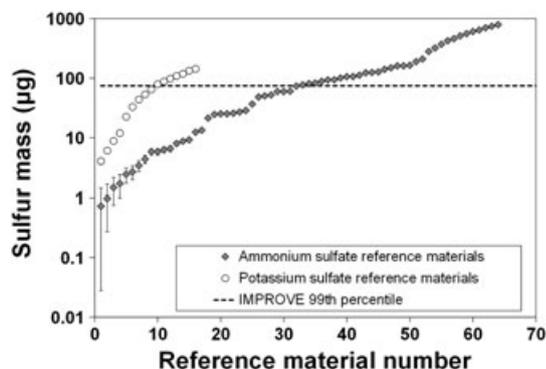
**Figure 3.** Sulfur mass of the 64 ammonium sulfate and 16 potassium sulfate reference materials. The mass uncertainty ( $0.7$  and  $0.5 \mu\text{g}$ , respectively) is given as vertical error bars. The IMPROVE measurement range for sulfur is shown by the horizontal dashed line as the 99th percentile value.
