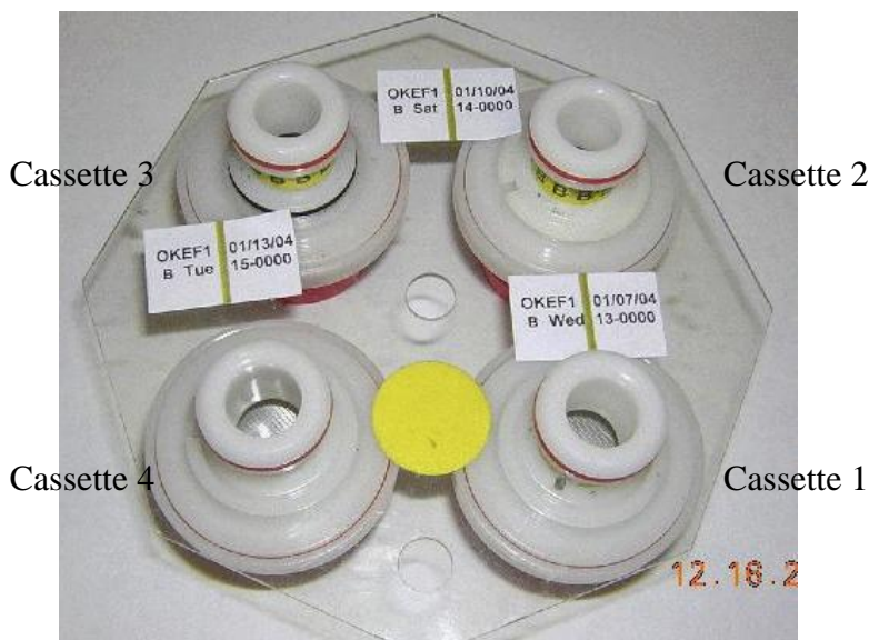
Figure 2-3. Sample cartridge for the B module (yellow sticker) with four cassettes. Only three of the cassettes contain sample filters (indicated by the three labels).
