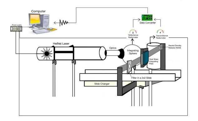
Figure 1. UC Davis Hybrid Laser Integrating Plate/Sphere (HIPS)
