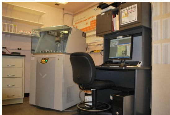
Figure 1. PANalytical Epsilon 5 analyzer and computer station in the XRF Laboratory at AQRC.
