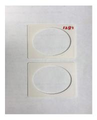
Next, place an unmarked slide on top of the filter and sandwich the filters using the slide press. Carefully lift the slide by the outer edge and make sure the slides are closed. If the slides are not fully closed then use the slide opener to gently open the slides and reseat the filter. Use the slide press to sandwich the filters.
