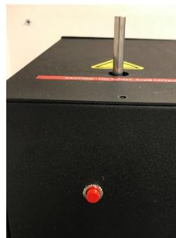
4. Push the red ignition button on the methanator to light the FID. A soft “pop” sound usually occurs with the FID lighting. Wait for the FID signal reading to increase above zero. If not, repeat the ignition.
