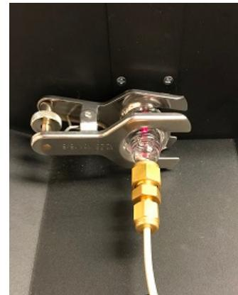
5. Use the silicone-coated forceps to *gently* slide the sample holder half way into the oven, then continue with the metal forceps until the sample holder is stopped by the tip of the oven thermocouple. Do not push the sample holder too hard or too fast, which could bend the thermocouple tip.
