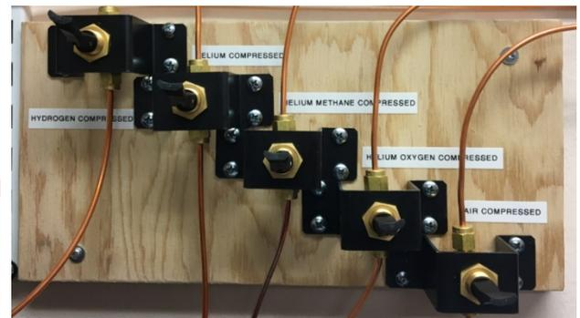
3. Turn the gas line valve to the “Closed” position (pointing down) for the gas to be changed.
