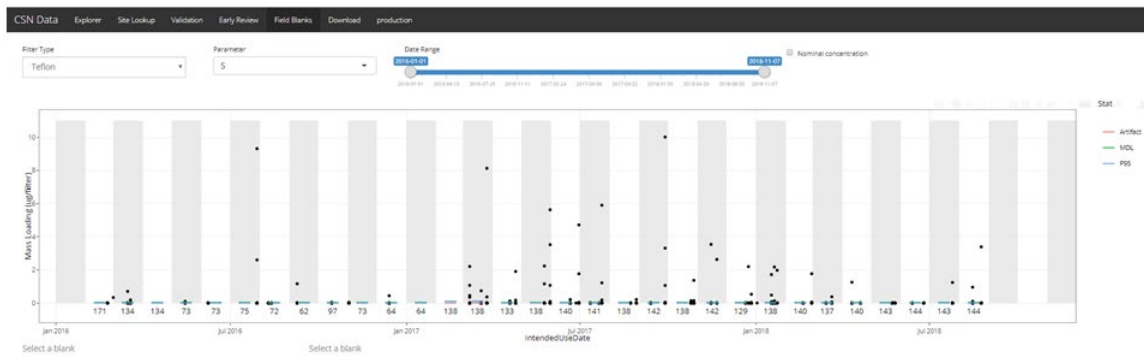
Figure 4. The Field Blanks tab of the CSN Data Explorer webapp showing the mass loading of a selected species from one of the three filter types for all field blank filters across the network.
