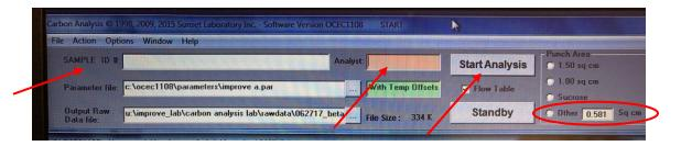
7. After finishing analysis of QC|QB, check Total Carbon (TC) concentration of "QC|QB" on the QC touchscreen. If  $TC \le 1.0 \,\mu\text{gC/cm}^2$ , proceed with running an instrument blank (QC|IB) without taking the filter punch out of the oven. Type in "QC|IB" in the Sample ID# box and select **Other 0.568 sq cm** (or the most updated punch area) as the punch area and click **Start analysis**. Otherwise, repeat the filter blank analysis with Sample ID
